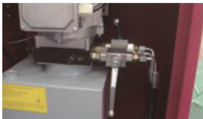
Main hose joint in the middle, and leveling hose joint on the each side
